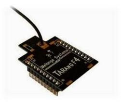
Fig 3.8 ZigBee Transceiver Model
