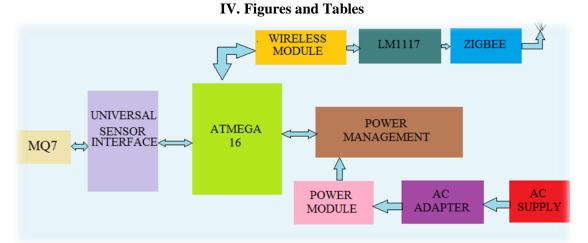
Figure.a. Transmitter Module
