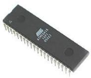
Fig 3.5 ATmega16 Microcontroller
