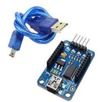
Fig 3.9 USB ZigBee Adapter
